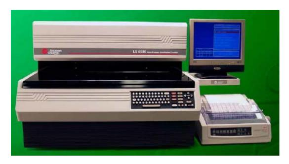
Figure 2.3-5. Photograph of the Beckman Coulter LS6500 multipurpose scintillation counter.
