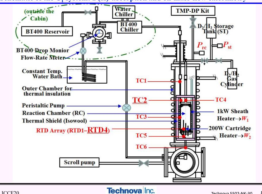
Schematic of the C<sub>1</sub> system: D(H)-absorption and oil-mass-flow calorimetry
