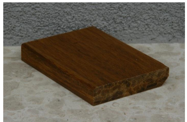
Photo 3.2.2: Example of high density strand woven bamboo fibre composite.
