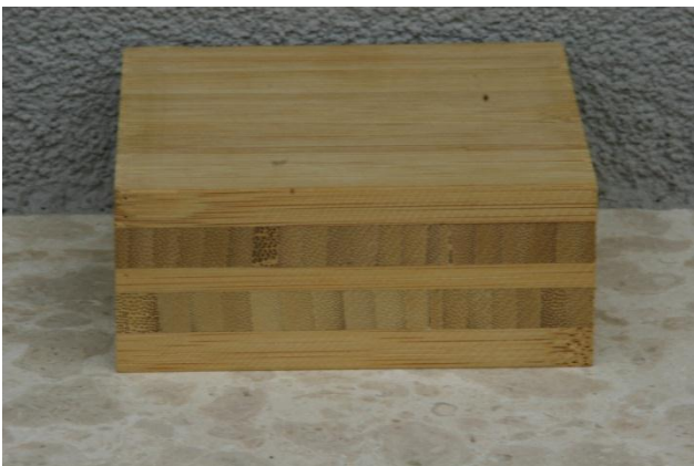
Photo 3.2.1: Example of 5-layered, vertical strips, bamboo plywood
