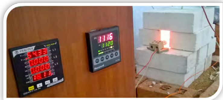
Fig2: Picture showing the reactor in operation along with the power and Temperature display
