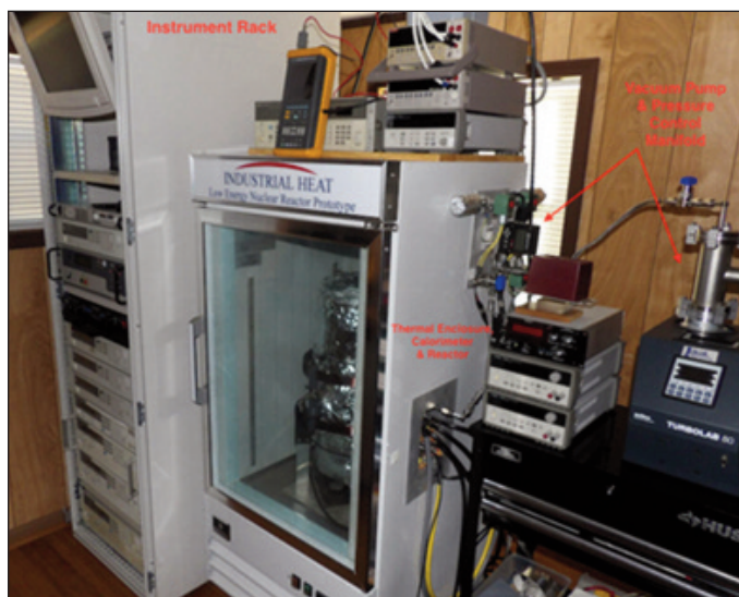
Figure 3. The setup in Letts lab, showing the instrumentation rack on the left, the thermal enclosure with the reactor in the center, and vacuum and other instrumentation on the right.
