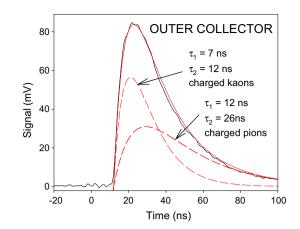
**Fig. 8** Signal at outer collector with bias -24 V with the coil in the beam in the same experiment as in Fig. 7. Note that the pions  $\pi^{\pm}$  have rise time of 12 ns equal to the decay time of the kaons K<sup>±</sup> as required for the decay chain K<sup>±</sup>  $\rightarrow \pi^{\pm} \rightarrow \mu^{\pm}$ . The actual signal is probably due to muons giving secondary electron ejection at collector
