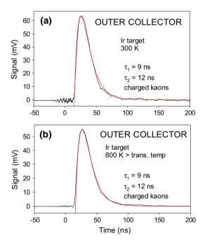
**Fig. 5** Charged kaon signal at the outer collector in Fig. 2 with bias -24 V. The meson signal exists even at a temperature of 800 K, above the D(0) on Ir transition temperature of 525 K [28]
