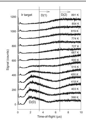
**Fig. 3** TOF spectra at  $45^{\circ}$  detector position relative to laser beam. D(0) on Ir surface. Temperature variation shown
