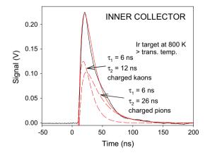
Fig. 6 Combined charged kaon and pion signal at the inner collector in Fig. 2 with bias -24 V. The meson signal exists even at a temperature of 800 K, above the D(0) on Ir transition temperature of 525 K [28]
