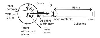
Fig. 2 Horizontal cut through the apparatus
