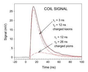
**Fig. 7** Current coil signal with D(0) on target. Coil at position of inner collector in Fig. 2. Note that the pions  $\pi^{\pm}$  have rise time of 12 ns equal to the decay time of the kaons  $K^{\pm}$  as required for the decay chain  $K^{\pm} \rightarrow \pi^{\pm} \rightarrow \mu^{\pm}$ . The actual particle current is probably due to muons
