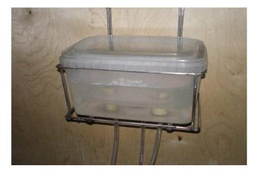
Figure 4: Water flow rate damping tank
