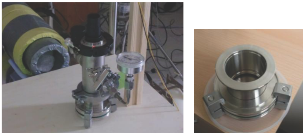
Figure 7. Photos of the reactor and the bottom part where the sample with the palladium film will be placed.
