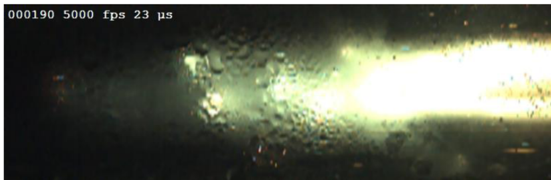
Figure 3. Frame of high-speed video. Exposure time is 20 \mu\text{s} . Right -cathode. Argon mass flow rate is 2 g/s and water vapour mass flow rate is 2 g/s.
