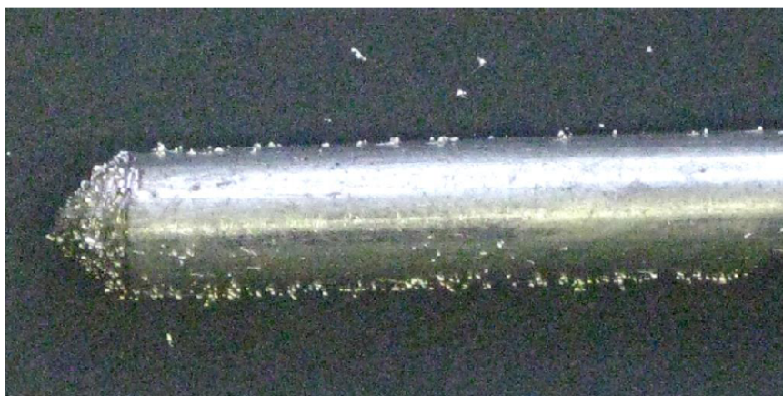
Figure 10. Anode surface is covered by tiny metal droplets injected from cathode. Cathode diameter is 5 mm .
