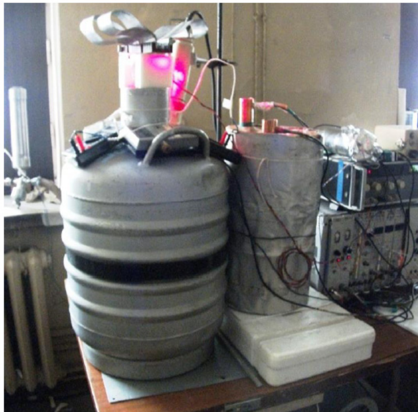
Figure 3. The experimental setup with an array of 9 LEDs and solution in the Dewar vessel.
